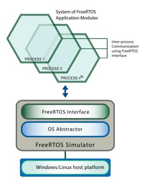
FreeRTOS Simulator provides the ability to simulate, test and run an entire system of C/C++ FreeRTOS applications on a Windows or Linux host. Host-based testing offers more hardware resources, less complexity and lower costs when compared to testing on a target platform. FreeRTOS Simulator provides the following features when used as a virtualized testing platform:
