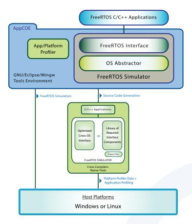
FreeRTOS Simulator is integrated with AppCOE, an Eclipse-based framework packaged with CDT, BIRT and GNU x86 tools, providing a state-of-the-art IDE for development and testing. FreeRTOS Simulator provides the following features when used as a development platform:
