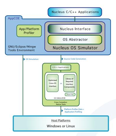
Nucleus OS Simulator is integrated with AppCOE, an Eclipse-based framework packaged with CDT, BIRT and GNU x86 tools, providing a state-of-the-art IDE for development and testing. Nucleus OS Simulator provides the following features when used as a development platform:
