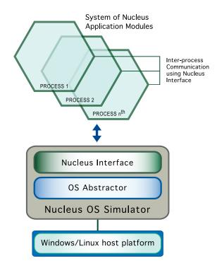
Nucleus OS Simulator provides the ability to simulate, test and run an entire system of C/C++ Nucleus applications on a Windows or Linux host. Host-based testing offers more hardware resources, less complexity and lower costs when compared to testing on a target platform. Nucleus OS Simulator provides the following features when used as a virtualized testing platform:
