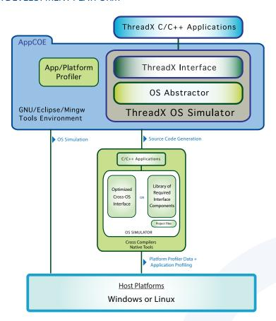
ThreadX OS Simulator is integrated with AppCOE, an Eclipse-based framework packaged with CDT, BIRT and GNU x86 tools, providing a state-of-the-art IDE for development and testing. ThreadX OS Simulator provides the following features when used as a development platform:
