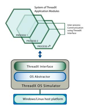
ThreadX OS Simulator provides the ability to simulate, test and run an entire system of C/C++ ThreadX applications on a Windows or Linux host. Host-based testing offers more hardware resources, less complexity and lower costs when compared to testing on a target platform. ThreadX OS Simulator provides the following features when used as a virtualized testing platform:
