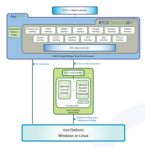
RTOS Simulator is integrated with AppCOE, an Eclipse-based framework packaged with CDT, BIRT and GNU x86 tools, providing a state-of-the-art IDE for development and testing. OS Simulator provides the following features when used as a development platform:
