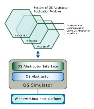
RTOS Simulator provides the ability to simulate, test and run an entire system of C/C++ OS Abstractor applications on a Windows or Linux host. Host-based testing offers more hardware resources, less complexity and lower costs when compared to testing on a target platform. RTOS Simulator provides the following features when used as a virtualized testing platform:
